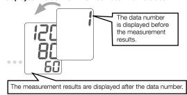
The value stored in memory is numbered in the order of measurements. For example, when 60 sets of data are stored in memory, the data number 1 represents the latest data.
